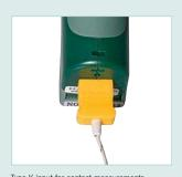
Type K input for contact measurements
